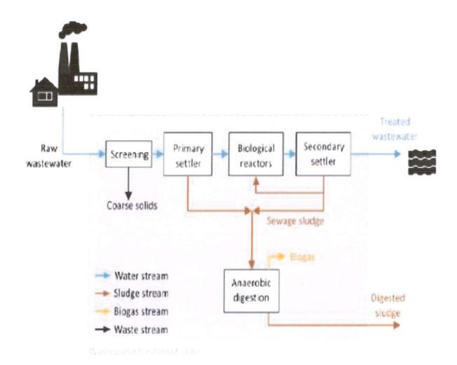
The physical process: this is the mechanical treatment of the water that involves removal of debris from the raw wastewater right from the point it enters the plant. The screening and primary settling of debris. Wastewater enters the treatment plant through the inlet chamber from where it is channeled to the coarse screen that removes solid waste.
